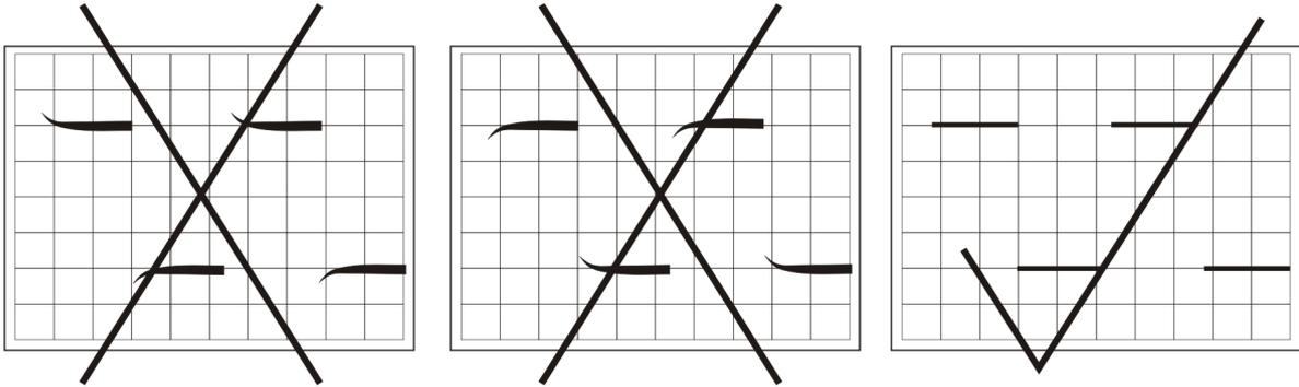
Illustration of 200Hz square wave adjustment.
